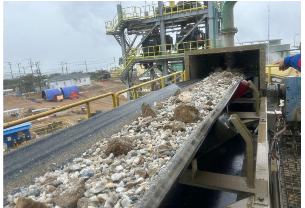
Figure 2. Conveyor to Transfer Crushed Ore to Sag & Ball Mill
