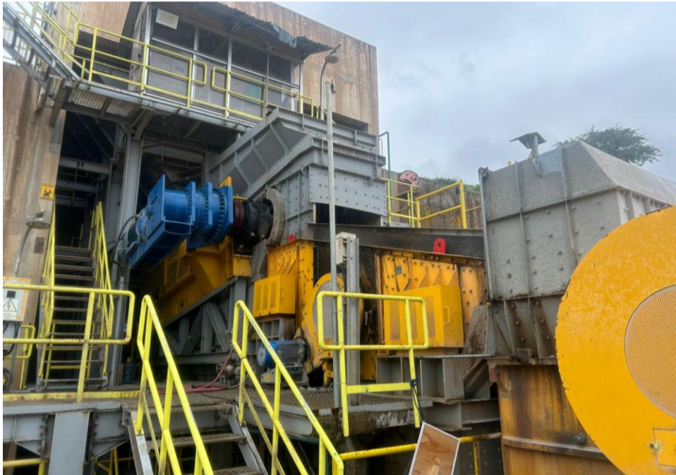
Figure 1. Jaw Crusher to Crush Mined Ore
