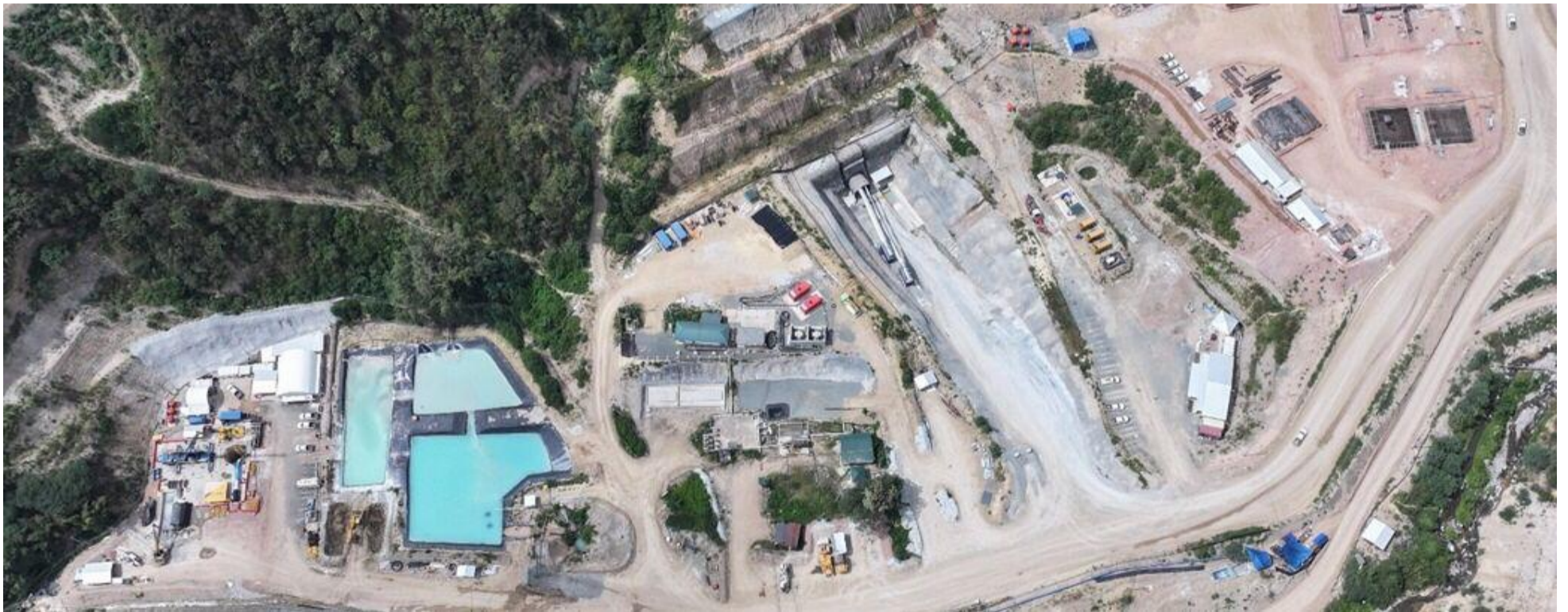
Figure 14. The view of the underground mine area from above (Portal to UG mine, UG tunnel, Paste Plant, Water Treatment area, Shaft Sink for air flow)
