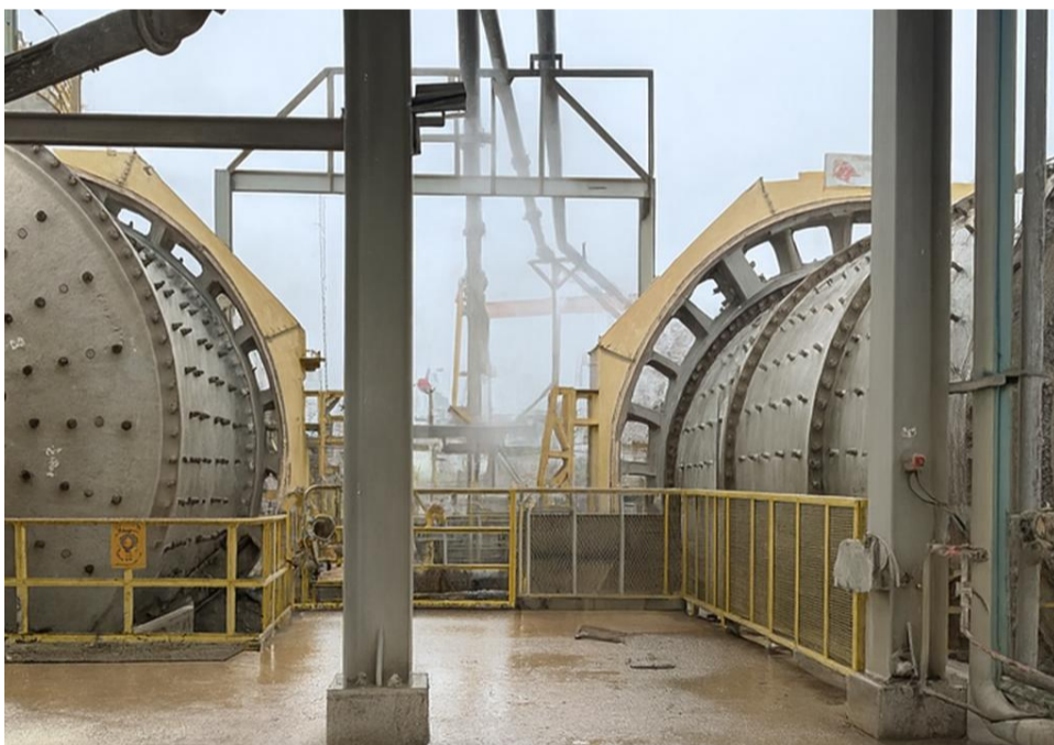
Figure 3. SAG and ball mills grind ore from ~12 mm to ~75 µm
